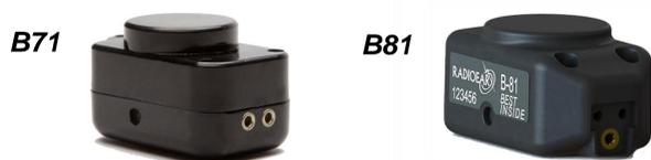
In an attempt to improve the low frequency performance, a new transducer principle called Balanced Electromagnetic Separation Transducer (BEST) was developed by Håkansson (2003). This is the motor unit used in the new B81 bone vibrator. Using the BEST™ principle, the static forces are counterbalanced so that non-linear distortion forces are reduced and maximum output levels can be increased.
