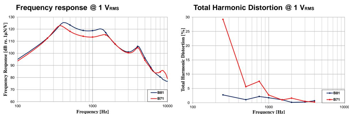
The frequency response of the B81 was designed to replicate the B71 and it was found that they were practically identical (median values of three devices) except for a small deviation at the mid frequencies where the B81 is more efficient (left). The THD was considerably lower for the B81 at low frequencies (right) when driven by a constant voltage of 1 V<sub>RMS</sub>.
